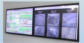
Subsystem of automatic scheduling and optimization. Tire operation accounting module. Tire pressure monitoring Remote diagnostics module. Maintenance and repair module Operating time module for main components and assemblies Integration module. Enterprise security service module
